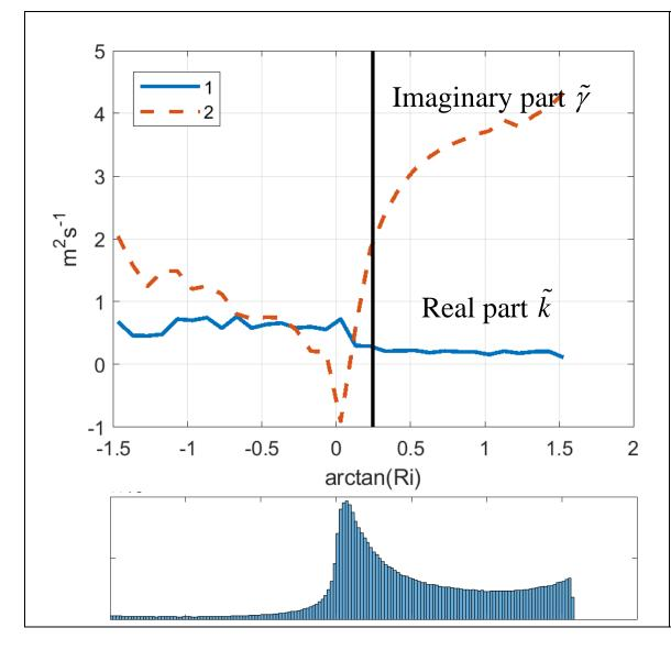
Optimal coefficients of turbulent exchange  $\tilde{\kappa}$  (Full subsample) depending on the  $S_3 = \arctan(Ri)$ , where Ri – Richardson number.
