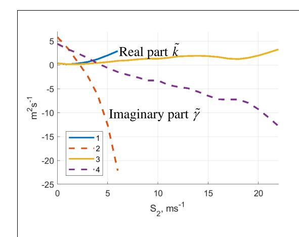
coefficient Optimal of turbulent exchange  $\tilde{\kappa}$  (full subsample): the real part  $\tilde{k}(S_2)$  (graphs 1, 3); the imaginary part  $\tilde{\gamma}(S_2)$  (graphs 2, 4) depending on the wind module shear  $S_2 = shear(z) = \sqrt{(u(z) - u_g)^2 + (v(z) - v_g)^2}$  $(m \cdot s^{-1})$ : for stable subsample (graphs 1, 2), for unstable subsample (graphs 3,4)
