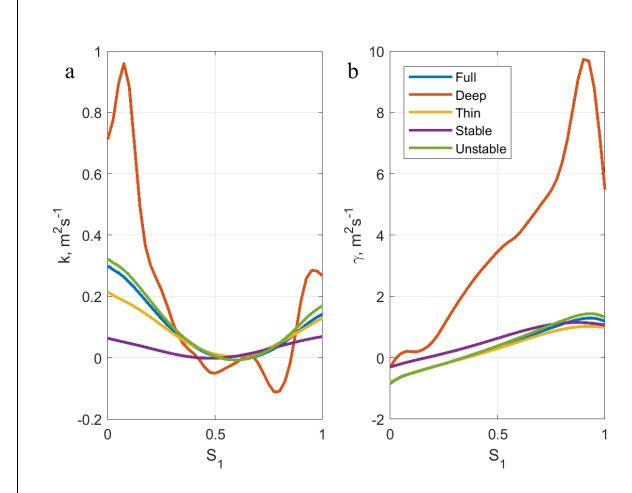
The optimal (for different subsamples) coefficient of turbulent exchange  $\kappa$  depending on the relative height  $S_1 = z/H$ :
