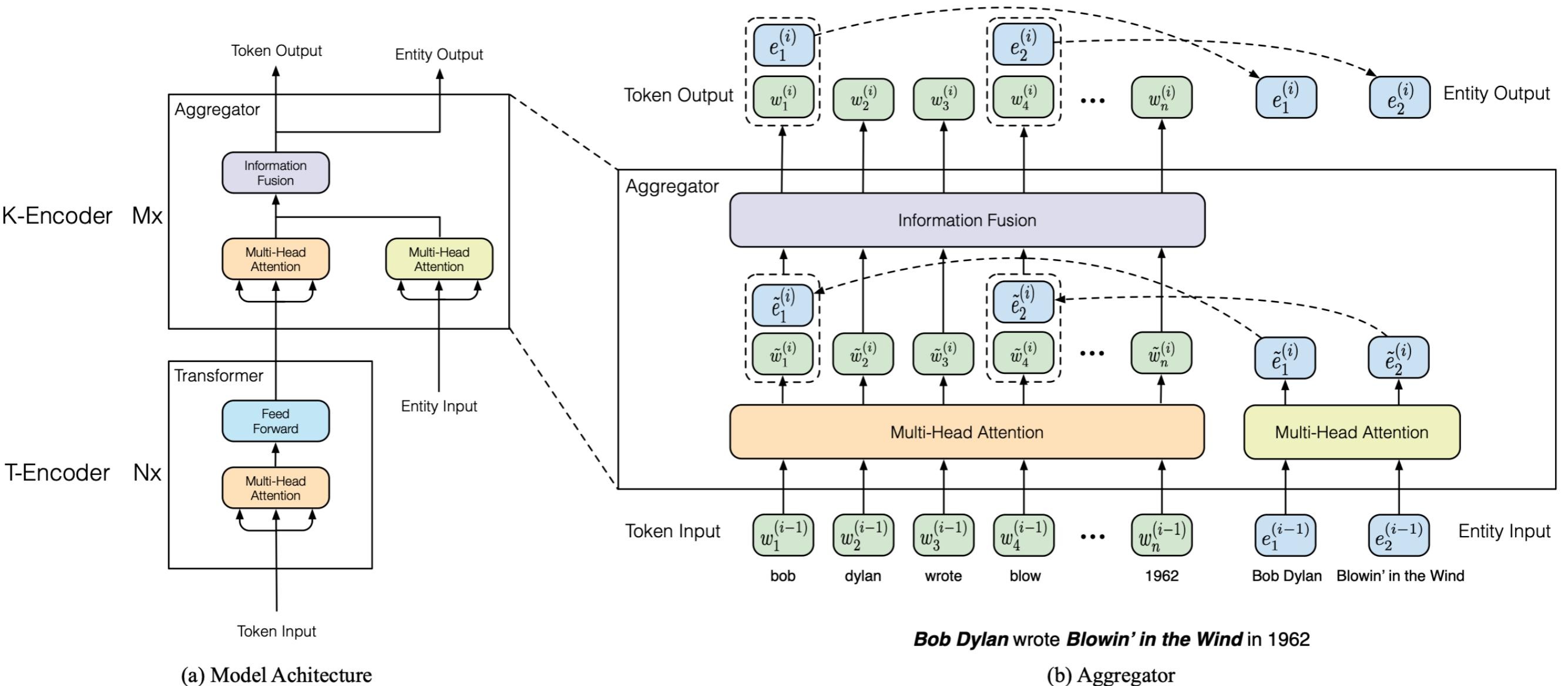
$$\begin{aligned}\{\tilde{\boldsymbol{w}}_1^{(i)},\ldots,\tilde{\boldsymbol{w}}_n^{(i)}\} &= \text{MH-ATT}(\{\boldsymbol{w}_1^{(i-1)},\ldots,\boldsymbol{w}_n^{(i-1)}\}), \\ \{\tilde{\boldsymbol{e}}_1^{(i)},\ldots,\tilde{\boldsymbol{e}}_m^{(i)}\} &= \text{MH-ATT}(\{\boldsymbol{e}_1^{(i-1)},\ldots,\boldsymbol{e}_m^{(i-1)}\}).\end{aligned}$$
