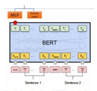
Figure 1: Setup for training a BERT domain classifier. Picture adapted from (Devlin et al., 2018)
