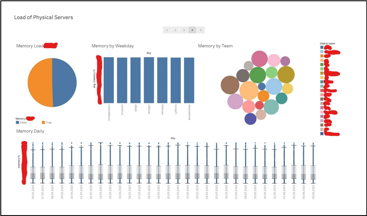
Figure 24. Number of servers using memory below a threshold, memory load weekly dynamics, average memory load by team, memory load dynamics throughout the observation period.
